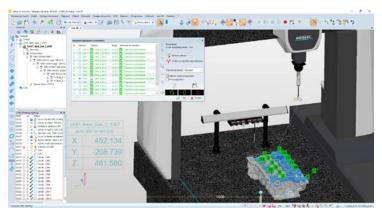
Path planning module for CMM. Optimized and collision-free path. Automatic head orientation. Real kinematic head replication.
