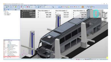
CMM quadriplex simulation with tool changer.
