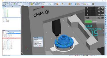
4-axis measurement simulation. CMM with rotary table using a touch probe.
