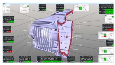
Silma takes advantage of extensive analysis capabilities from X4 software foundation. Embedded GD&T within CAD file.
