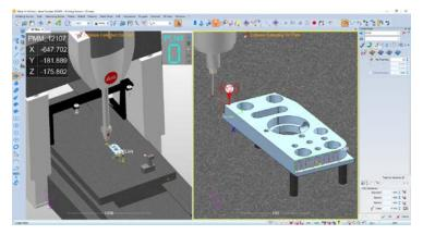
CMM with moving table. Inspection path creation with collision detection and automatic avoidance.
